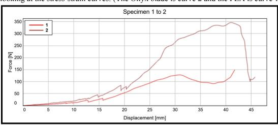
The instron tests yielded some interesting results, and we can extract information just by looking at the stress-strain curves: (The Onyx blade is curve 2 and the PLA is curve 1.)
